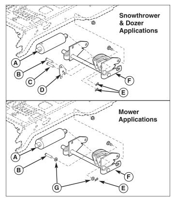
Figure 28. Lift Lock Plate - Hydraulic Lift Models
